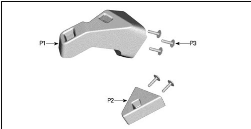
**NOTE:** Kit (P/N 295100948) is used on LH side, while kit (P/N 295100949) is used on RH side.
